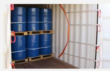
In addition, sheet restraint systems prevent slipping of the goods into the door of the container, thus avoiding accidents when opening the container doors.
