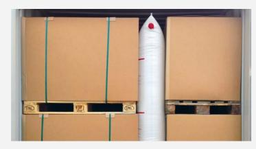
These must be closed in order to stop the goods and pallets from shifting due to the forces at work during overseas shipping or similar.
